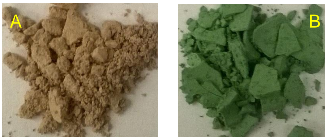
Figure 14. Microscope photographs of bulk precipitate of Ni(PiPCO) 2 ·2H 2 O (A) and Cu(PiPCO) 2 ·H 2 O (B), taken at x40 magnification.
