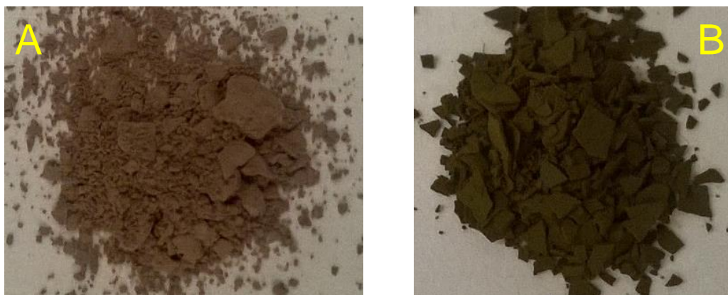
Figure 12. Microscope photographs of bulk Precipitate of Ni(PyrCO) 2 ·2H 2 O (A) and Cu(PyrCO) 2 ·H 2 O (B) at x40 magnification.
