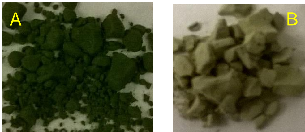
Figure 8. Microscope photographs of bulk precipitate of Ni(PiCO) 2 ·H 2 O (A) and Cu(PiCO) 2 (B) obtained at 40x magnification.
