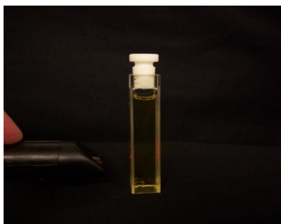
Figure 8: Actual photographs of \text{Pt}(\text{MCO})_2 in solutions. (A): the Tyndall effect in aggregated opalescent green solutions of \text{Pt}(\text{MCO})_2 in DMF showing significant light scattering; B – the monomeric species of \text{Pt}(\text{MCO})_2 in the same solution after addition of DMSO.
