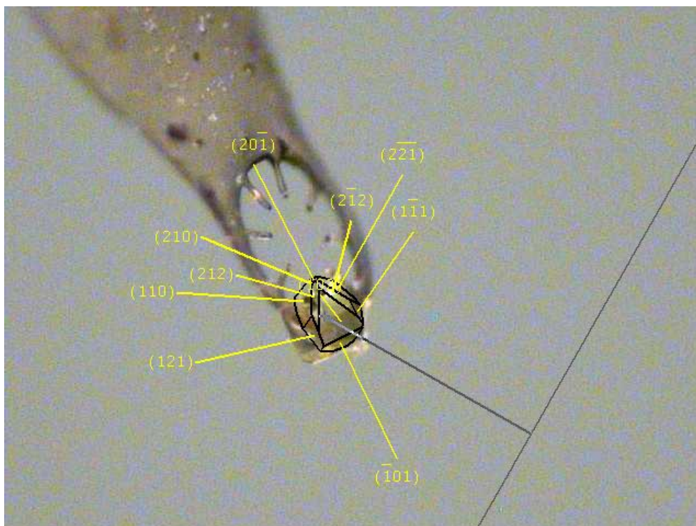
Figure 42. Video microscope image of the crystal of Sb(Ph)_4(TCO) , polymorph 1 , with indexed faces.
