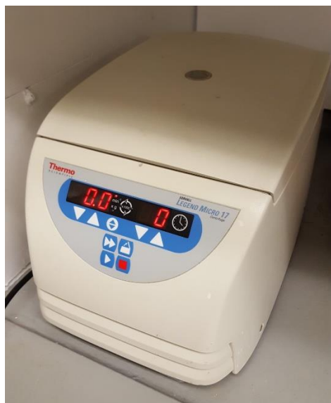
Figure 17. Instrumentation and accessories used for isolation of organoantimony(V) cyanoximates from Ag(I)Br. A Thermo Scientific centrifuge (left) with filtered nylon Eppendorf tubes (right).
