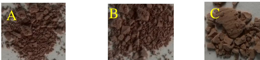
Figure 42. The microscope photographs of the hydrated \text{Ni}(\text{PyrCO})_2 \cdot 2\text{H}_2\text{O} (A), anhydrous \text{Ni}(\text{PyrCO})_2 (B) and rehydrated \text{Ni}(\text{PyrCO})_2 \cdot 2\text{H}_2\text{O} (C) at x40 magnification.
