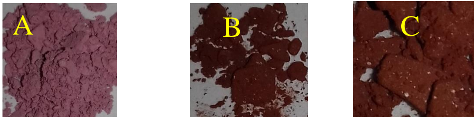
Figure 39. The microscope photographs of the hydrated \text{Ni}(\text{2PCO})_2 \cdot 2\text{H}_2\text{O} (A), anhydrous \text{Ni}(\text{2PCO})_2 (B) and rehydrated \text{Ni}(\text{2PCO})_2 \cdot 2\text{H}_2\text{O} (C) complex at x40 magnification.
